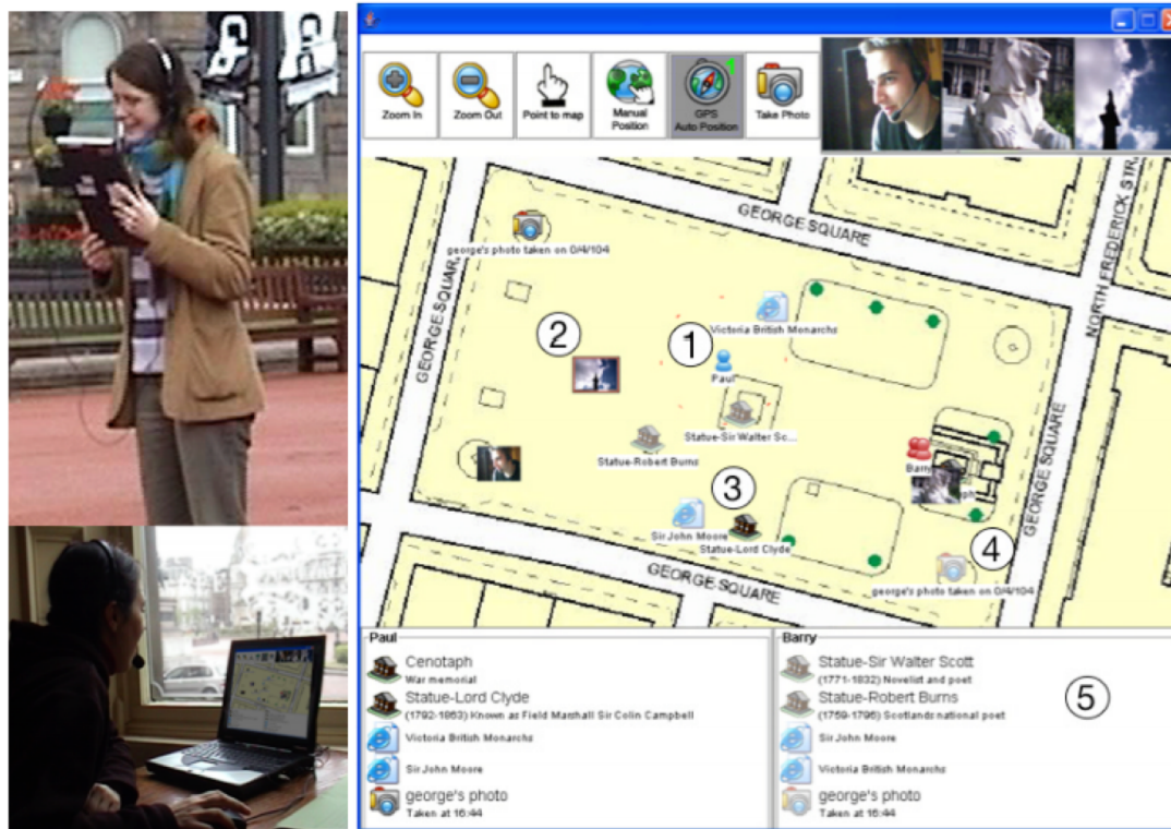
Figure 1. Example usage of the system and screenshot showing a map that displays each user's location (1), thumbnail photos (2), recommended locations, web pages (3) and photos (4), and each user's recommendation list (5).
